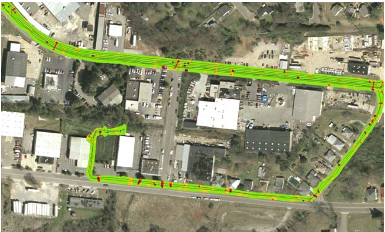
GEM-3 Array data obtained along streets in Raleigh, NC, superimposed upon an aerial photograph of the area. The survey was undertaken to detect all utility lines (water, sewer, powerline, telephone and fiber optic cables) buried under the road. Faint black lines indicate the ground track of the array.
