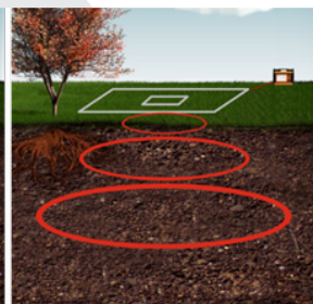
The collapsing magnetic field creates electrical currents in the ground
