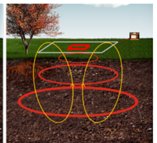
Ground currents create a secondary magnetic field recorded by the RX loop
